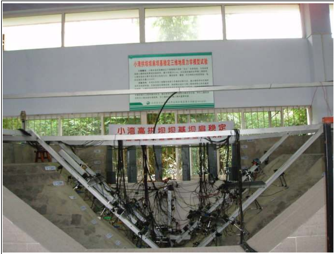
A5: Model of dam was tested in Sichuan University.
