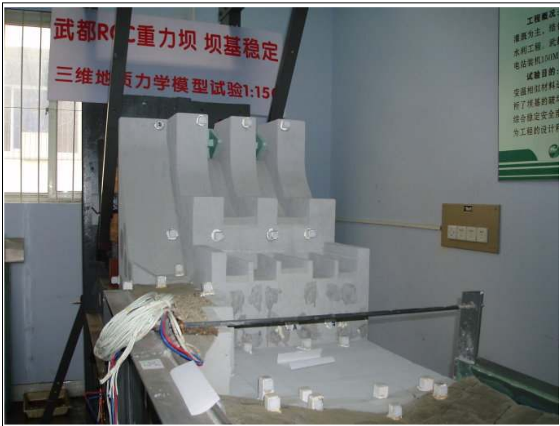
A4: Model of dam was tested in Sichuan University.
